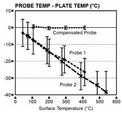
Figure 3. A Comparison Between The Thermally Compensated Probe & Two Standard Probes.
